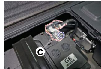
3-3. Turn the ignition switch OFF and disconnect the auxiliary 12V auxiliary battery negative (-) terminal (C).
