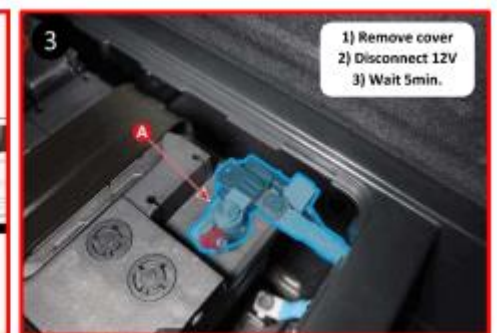
3-3. Turn the ignition switch OFF and disconnect the auxiliary 12V auxiliary battery negative (-) terminal (C).
